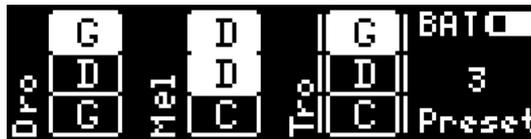
Fig. 12: The home screen in 9 Strings, grouped by number mode with the trompette set active
