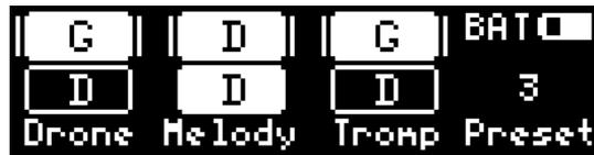
Fig. 3: The home screen in 6 String mode with the first string set active
