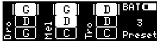
Fig. 6: The home screen in 9 Strings, grouped by number mode with the first string set active
