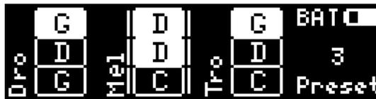
Fig. 11: The home screen in 9 Strings, grouped by number mode with the melody set active
