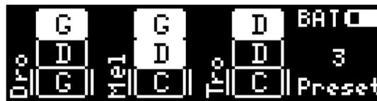
Fig. 8 – The home screen in 9 Strings, grouped by number mode with the third string set active
