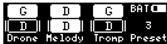
Fig. 4 – The home screen in 6 String mode with the second string set active
